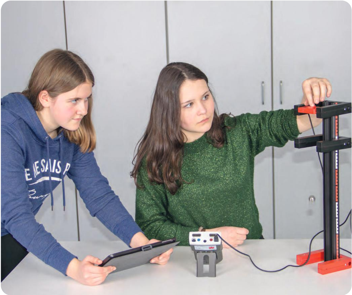
LP1.3.4.1C Determining the acceleration of gravity by plotting a s(t) diagram
