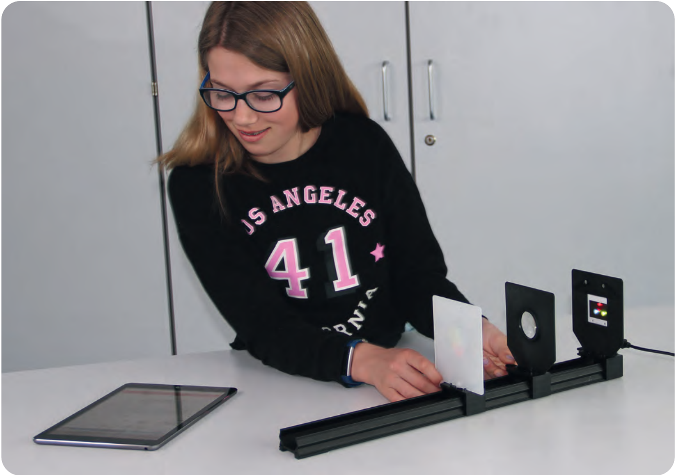
LP5.2.3.4 Additive mixing of three light colours
