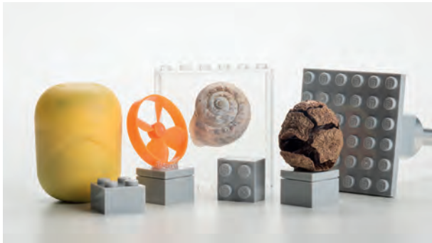
Various objects for a computed tomography, which can simply be attached to the LEGO adapter.
