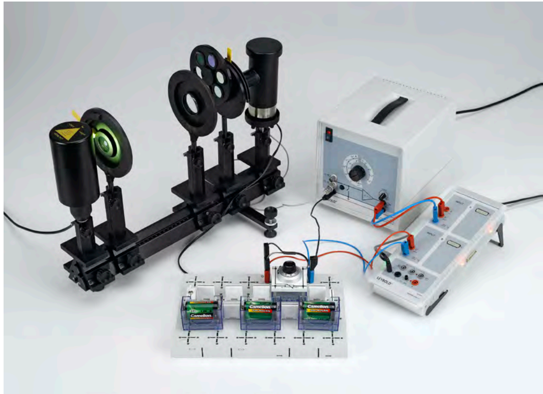
Determining Planck's constant - Recording the current-voltage characteristics, selection of wavelengths using interference filters on the optical bench (P6.1.4.4)
