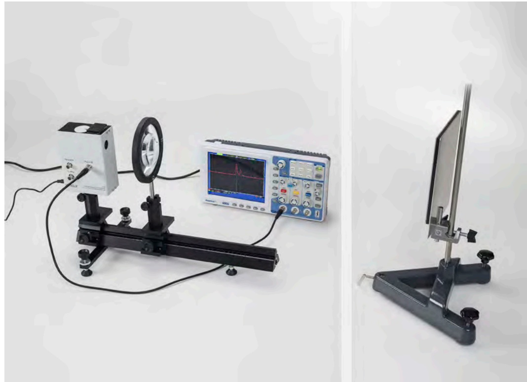
Determining the velocity of light in air from the path and transit time of a short light pulse (P5.6.2.1)
