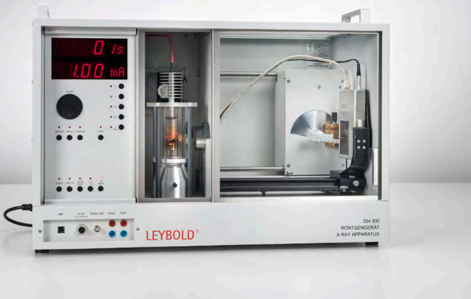
Measurement and presentation of a computed tomogram with the X-ray image sensor (P6.3.8.11)
