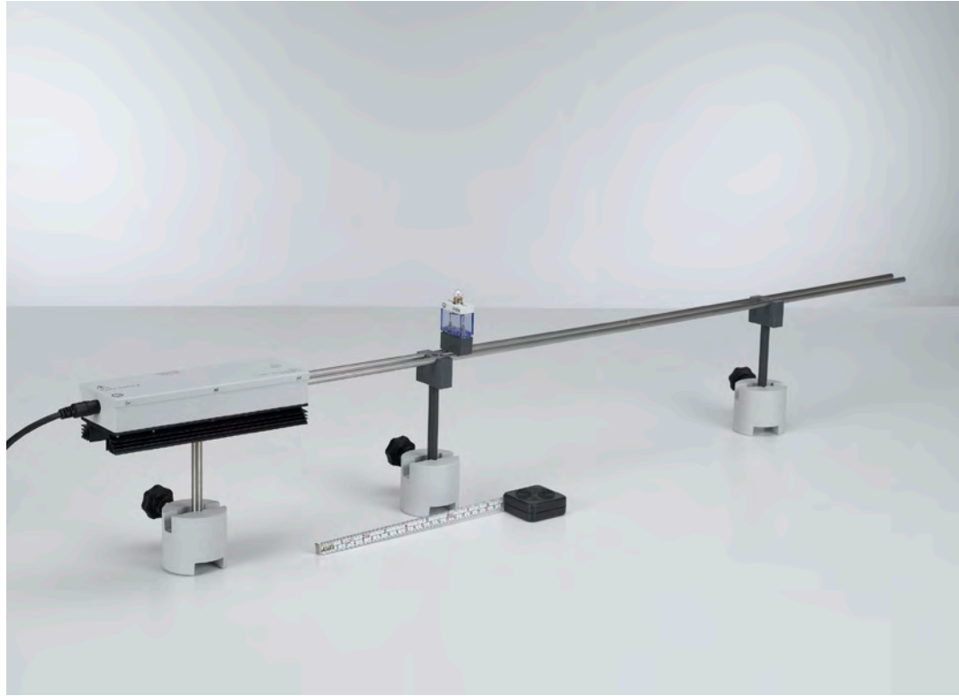
Determining the current and voltage maxima on a Lecher line (P3.7.3.1)
