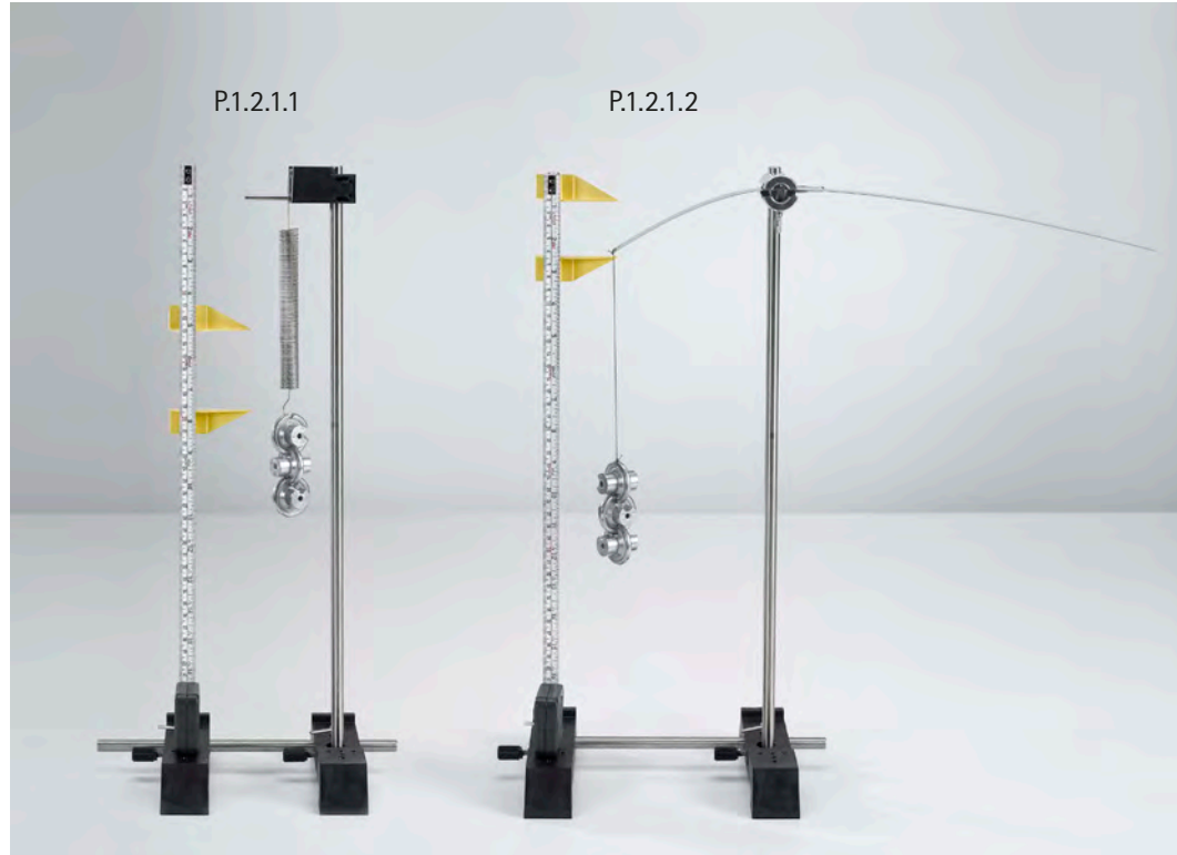
Expansion of a helical spring (P1.2.1.1)
