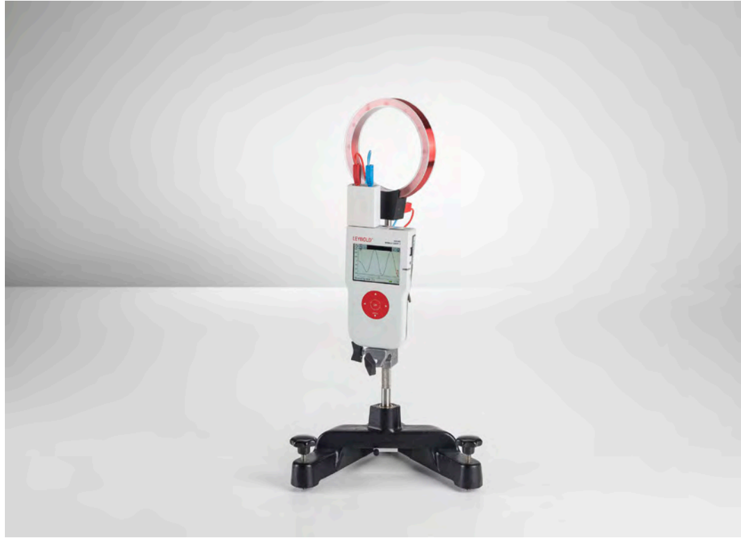
Measuring the earth's magnetic field with a rotating induction coil and CASSY (P3.4.6.2)
