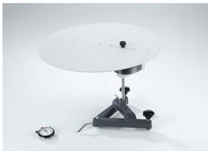
Confirming Steiner's theorem (P1.4.5.3)
