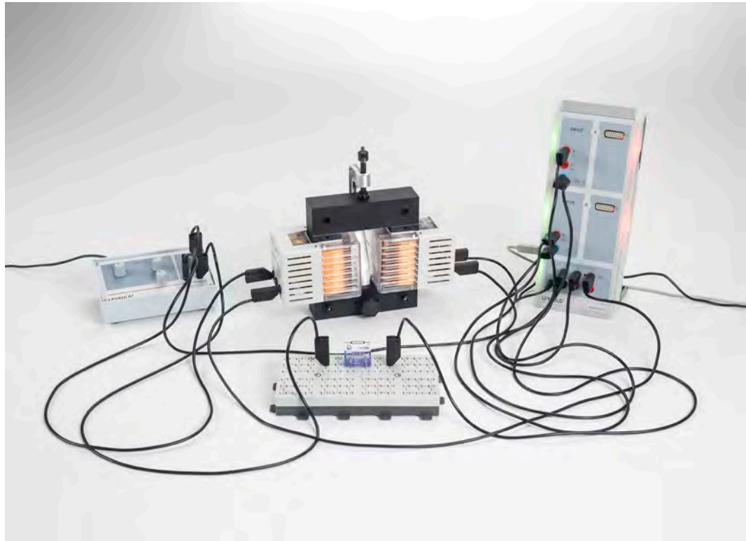
Recording the initial magnetization curve and the hysteresis curve of a ferromagnet and iron (P7.3.2.1)
