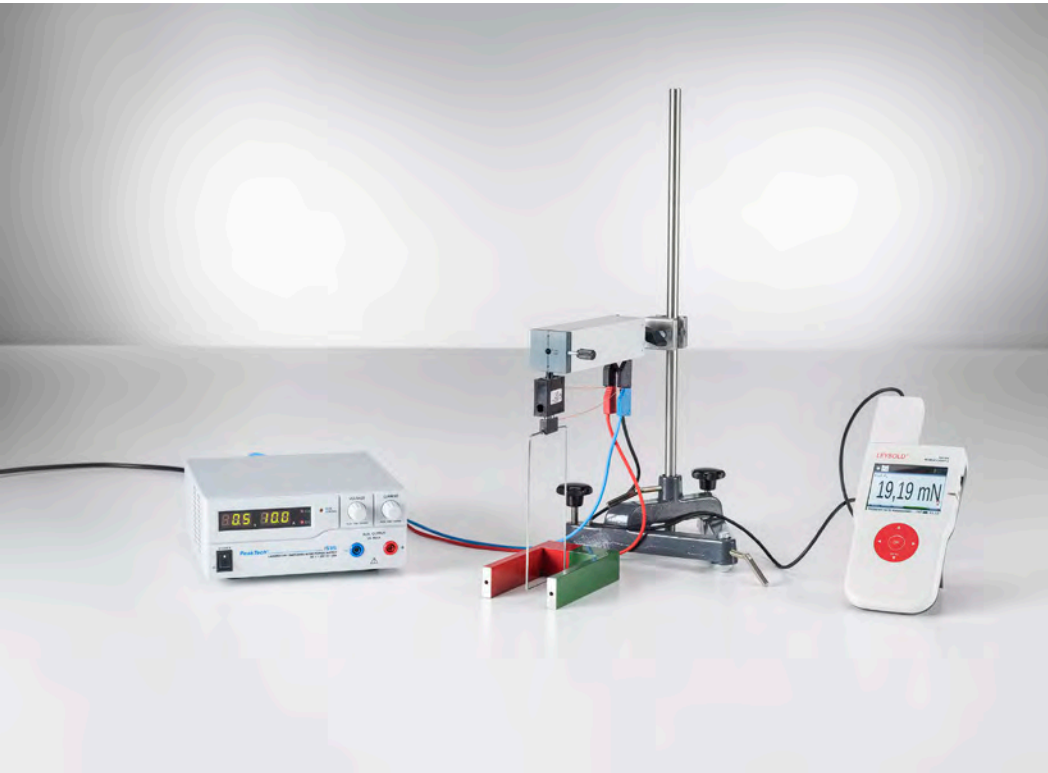
Measuring the force acting on current-carrying conductors in the field of a horseshoe magnet (P3.3.3.1)
