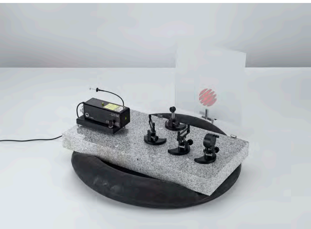
Determining the wavelength of the light of an He-Ne laser using a Fabry-Perot interferometer (P5.3.5.3)
