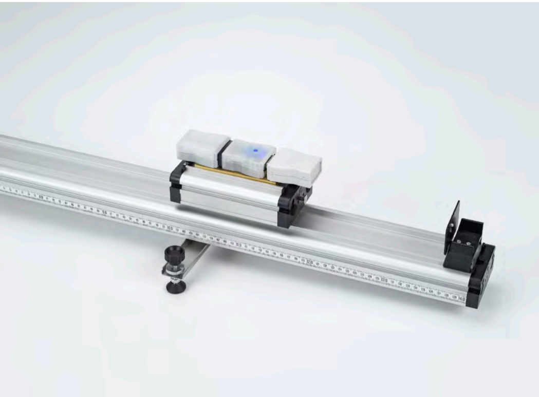
Accelerated motions with an acceleration sensor (P1.3.2.5)
