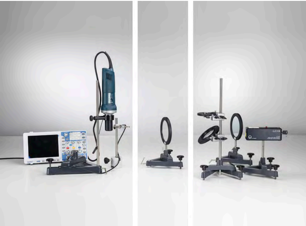
Determining the velocity of light by means of the rotating-mirror method according to Foucault and Michelson - Measuring the image shift as a function of the rotational speed of the mirror (P5.6.1.1)
