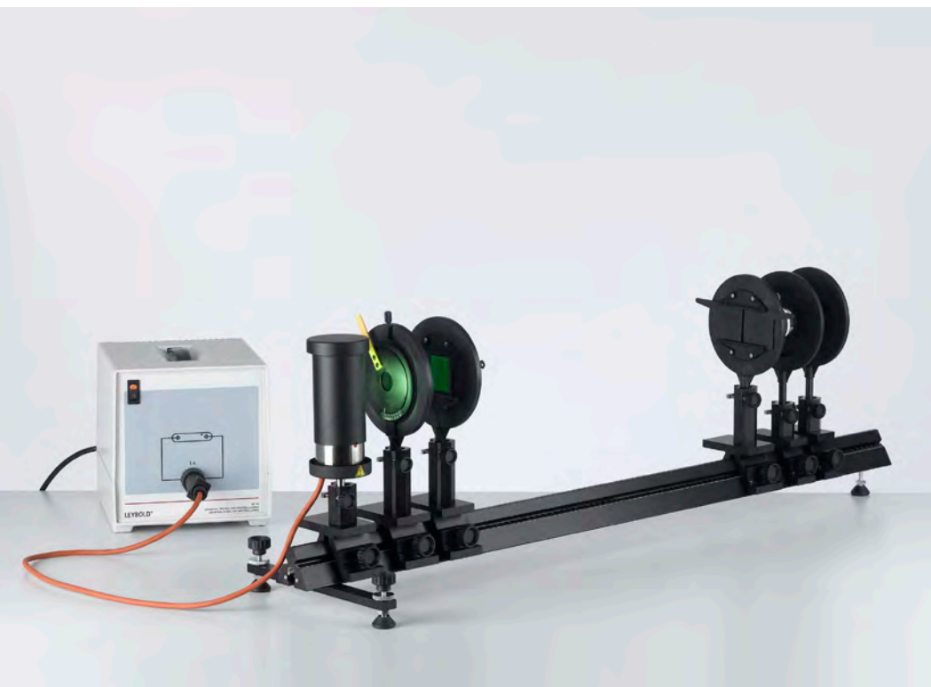
Investigation of the spatial coherence of an extended light source (P5.3.1.9)
