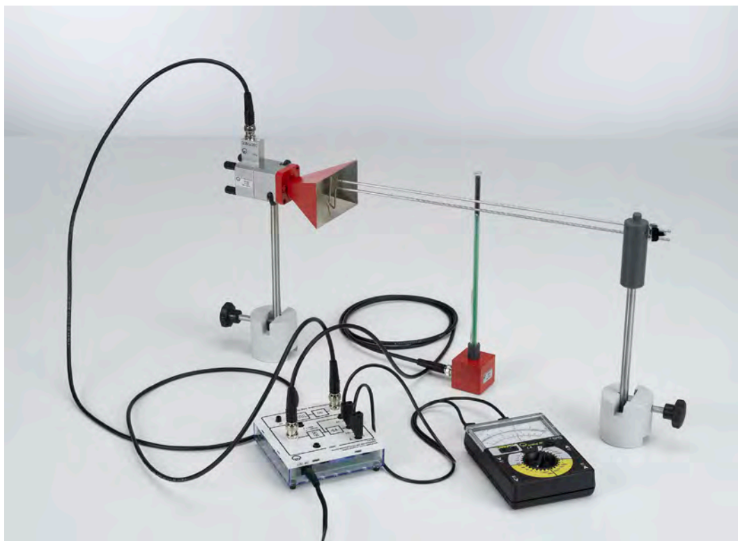
Guiding of microwaves along a Lecher line (P3.7.5.1)
