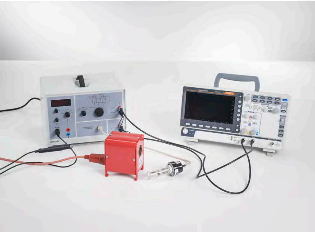
Franck-Hertz experiment with mercury - Recording with the oscilloscope (P6.2.4.1)
