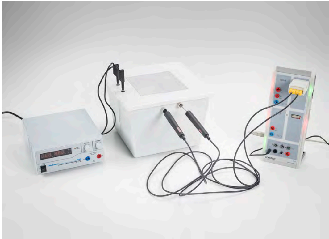
Determining the thermal conductivity of building materials using the single-plate method (P2.2.1.1)
