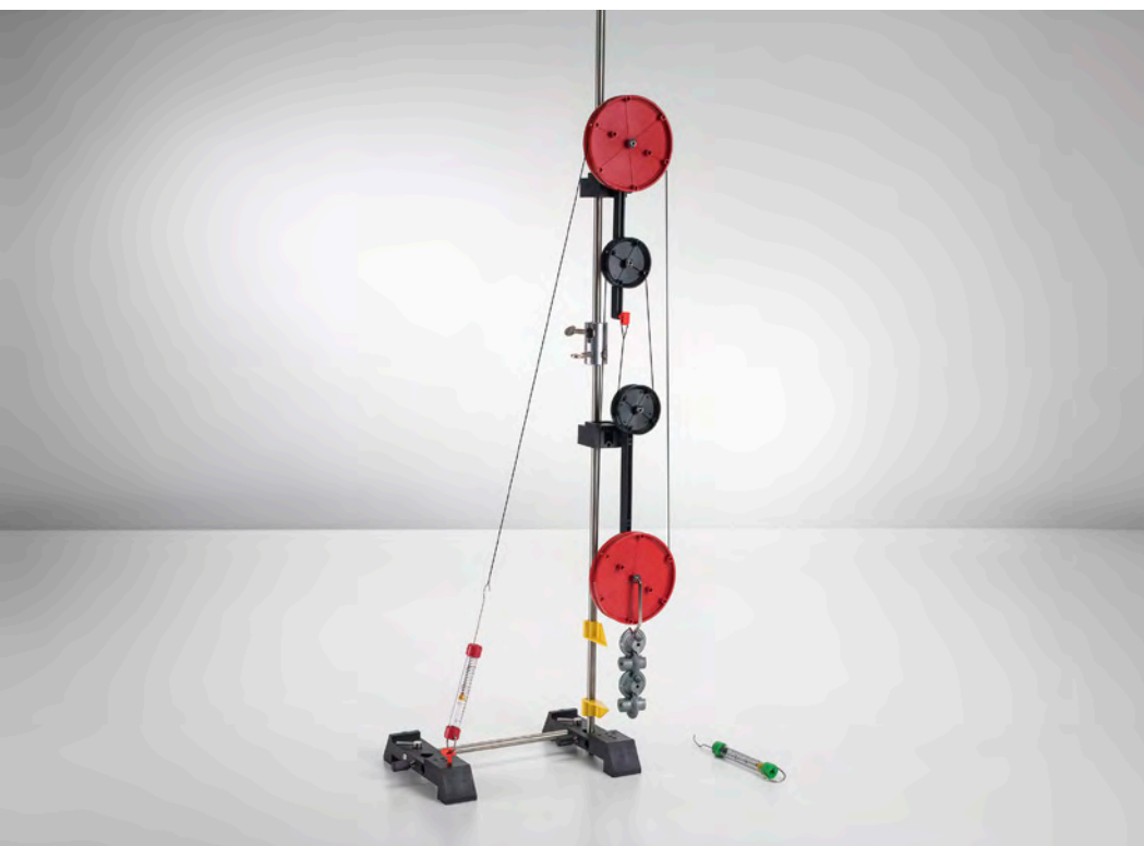
Fixed pulley, loose pulley and block and tackle as simple machines (P1.2.4.1)
