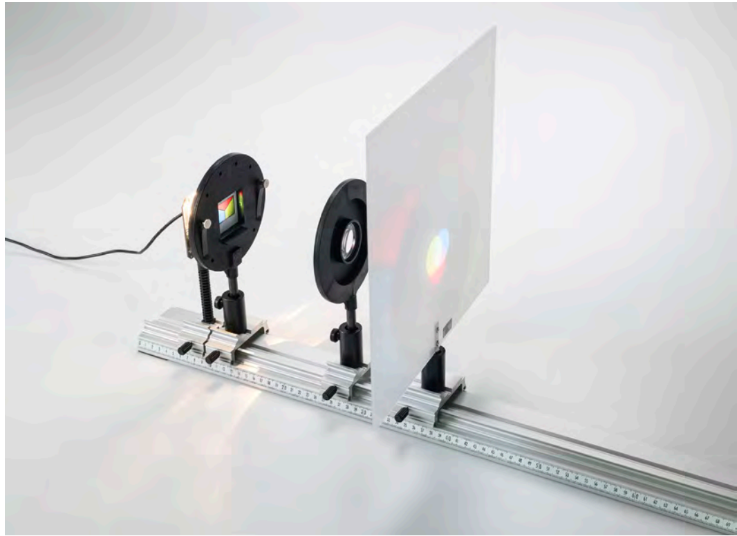
Demonstration of additive color mixing (P5.2.3.2)
