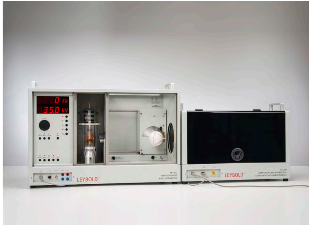
Measurement and presentation of a computed tomogram with the computed tomography module (P6.3.8.1)
