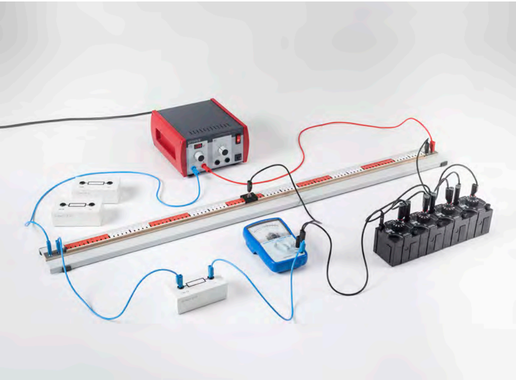
Determining resistances using a Wheatstone bridge (P3.2.3.4)
