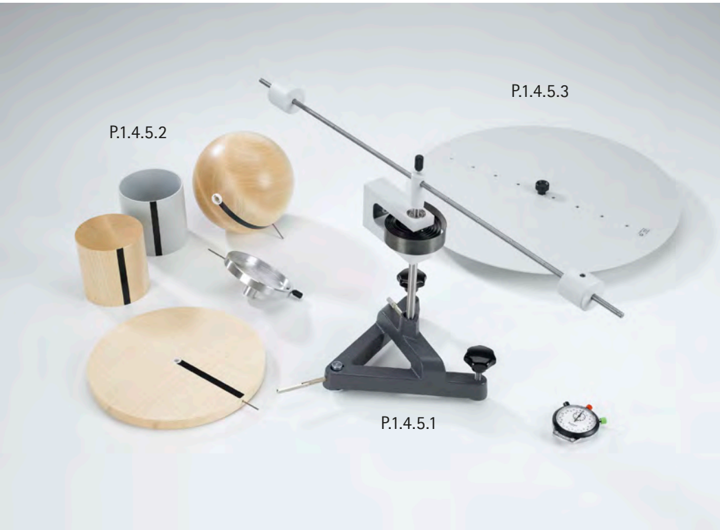
Definition of moment of inertia (P1.4.5.1)
