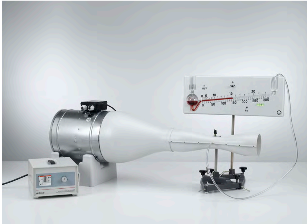
Static pressure and determination of the volume flow with a Venturi tube - Measuring the pressure with the precision manometer (P1.8.5.1)
