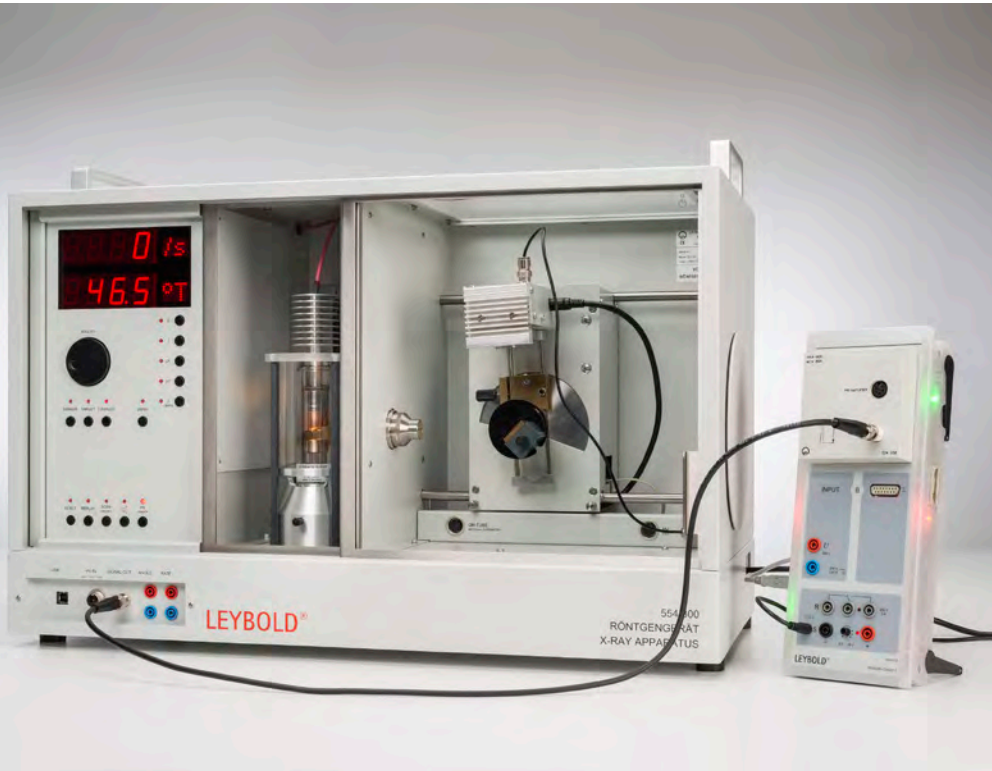
Application of X-ray fluorescence for the non-destructive analysis of the chemical composition (P7.5.1.1)
