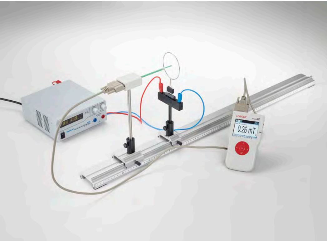
Measuring the magnetic field for a straight conductor and on circular conductor loops (P3.3.4.1)
