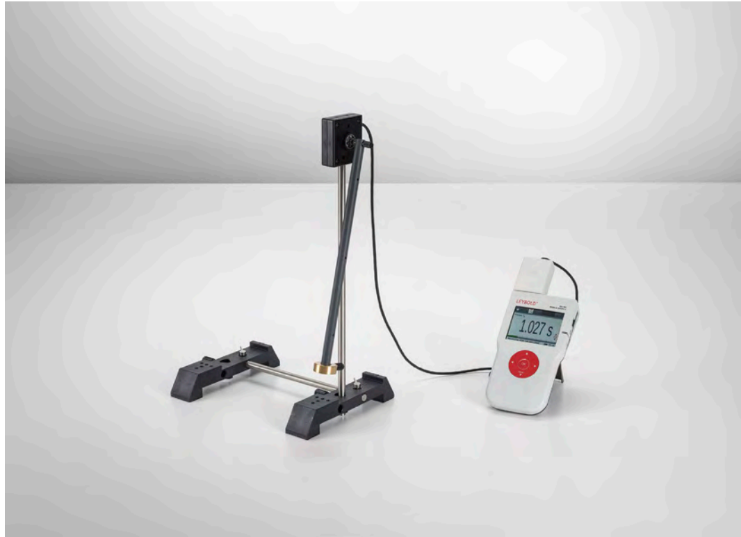
Oscillations of a rod pendulum and determination of the acceleration due to gravity on earth - Measuring with rotary motion sensor (P1.5.1.3)
