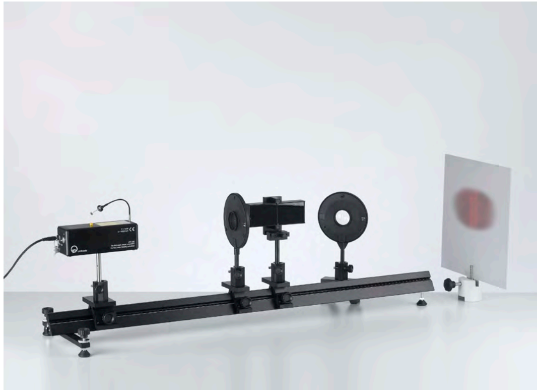
Interference at a Fresnel's mirror with an He-Ne laser (P5.3.2.1)
