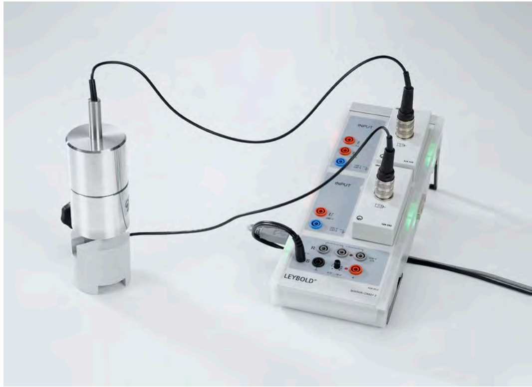
Detection of Muons (P6.6.2.1)
