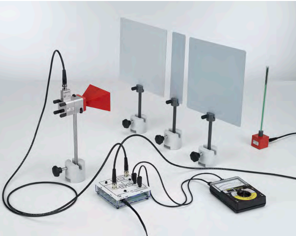
Diffraction of microwaves (P3.7.4.4)
