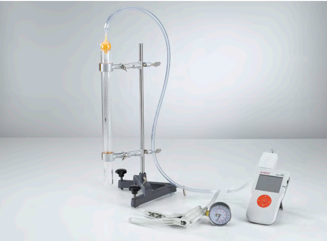
Pressure-dependency of the volume of a gas at a constant temperature (Boyle-Mariotte's law) (P2.5.2.1)
