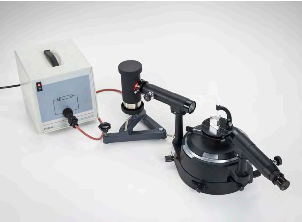
Measuring the line spectra of inert gases and metal vapors using a prism spectrometer (P5.7.1.1)
