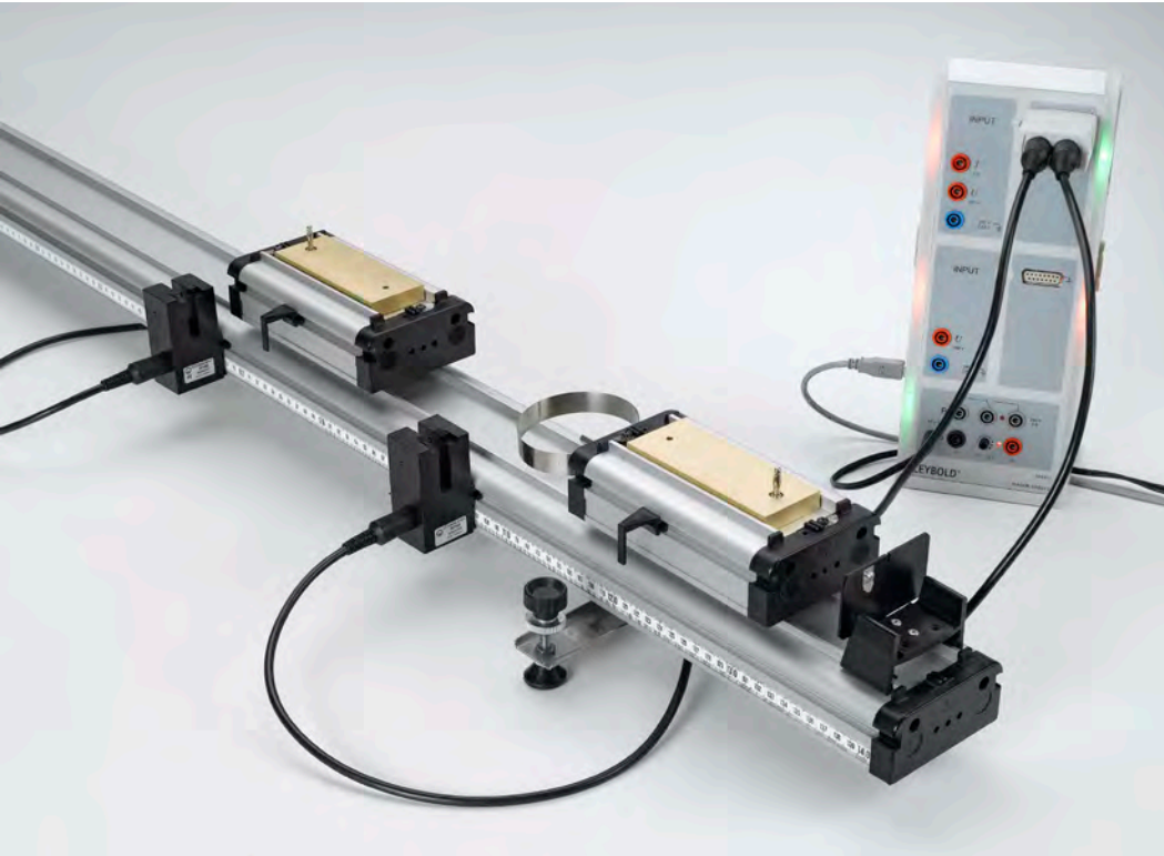
Energy and linear momentum in elastic and inelastic collision with Fletcher's trolleys - Measuring with two forked light barriers and CASSY (P1.3.4.1)
