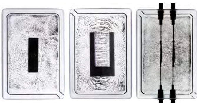
Displaying lines of magnetic flux (P3.3.1.1)
