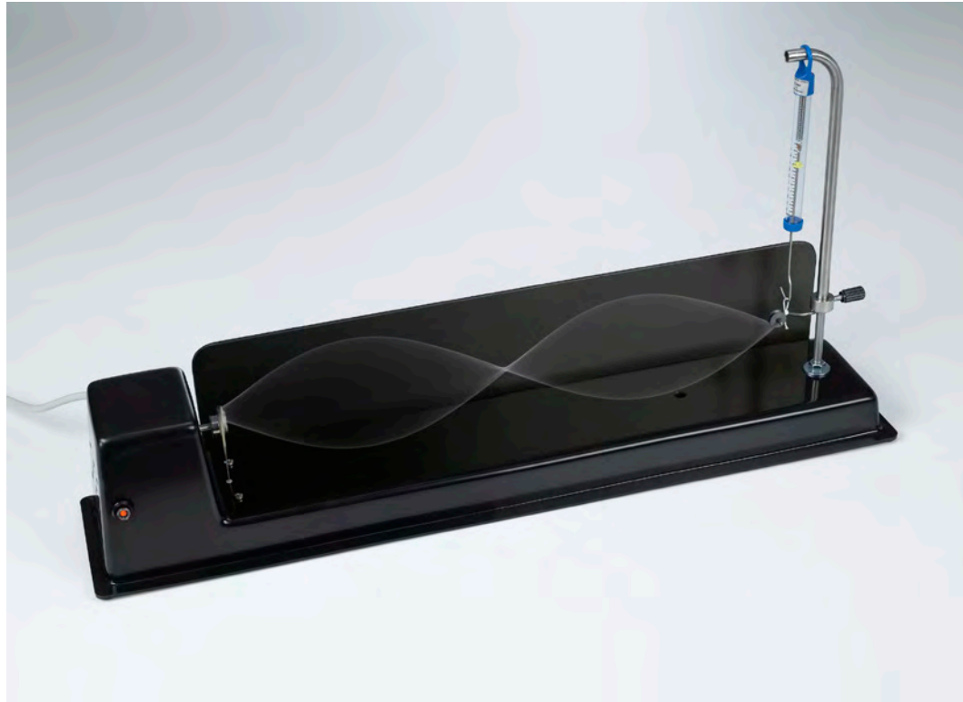
Investigating circularly polarized string waves in the experiment setup according to Melde (P1.6.3.1)
