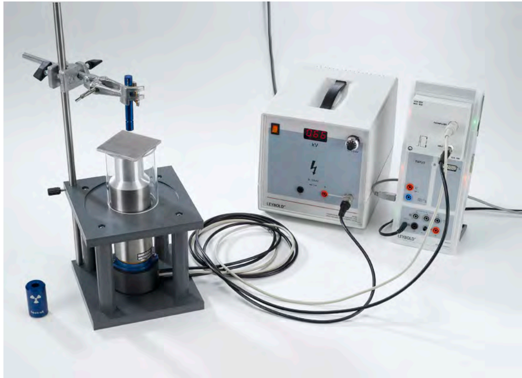
Absorption of \gamma radiation (P6.5.5.3)
