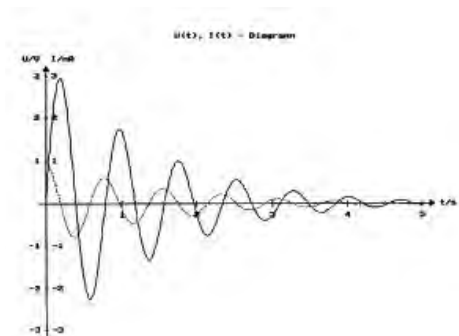
Damped electromagnetic oscillation in the 1 Hz range (P3.7.1.1)
