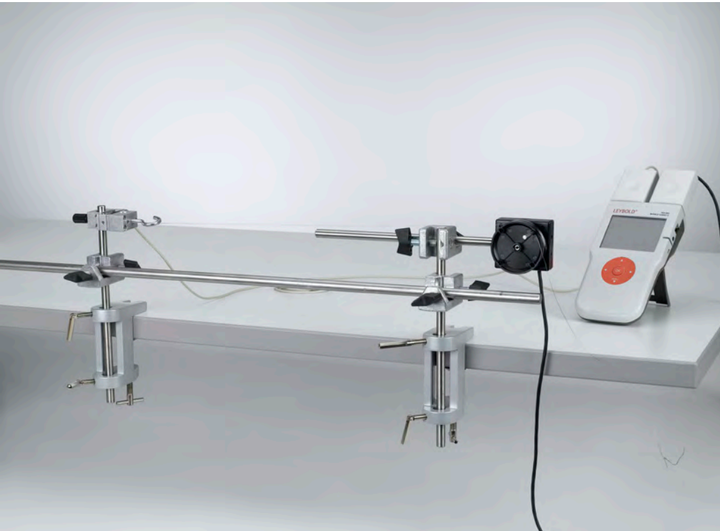
Investigating the elastic and plastic extension of metal wires - Recording and evaluating with CASSY (P7.1.4.2)
