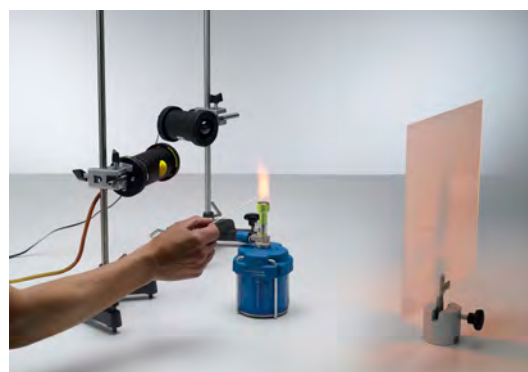
Qualitative investigation of the absorption spectrum of sodium (P6.2.2.2)
