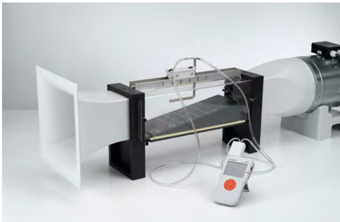
Verifying the Bernoulli equation - Measuring with a pressure sensor and Mobile-CASSY (P1.8.7.4)
