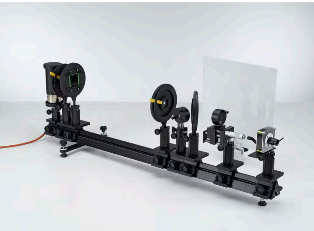
Determination of the coherence time and the line width of spectral lines with the Michelson interferometer (P5.3.4.4)
