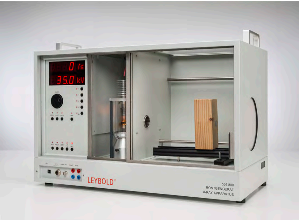
Investigation of an implant model (P6.3.1.5)
