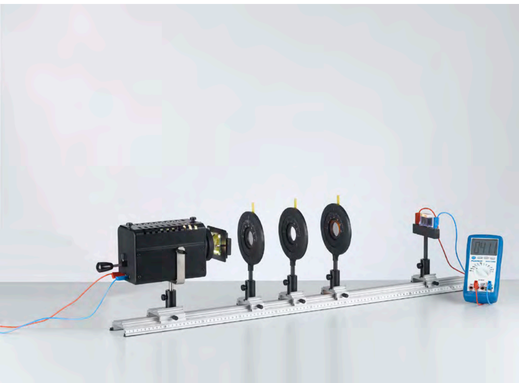
Quarter-wavelength and half-wavelength plate (P5.4.2.2)
