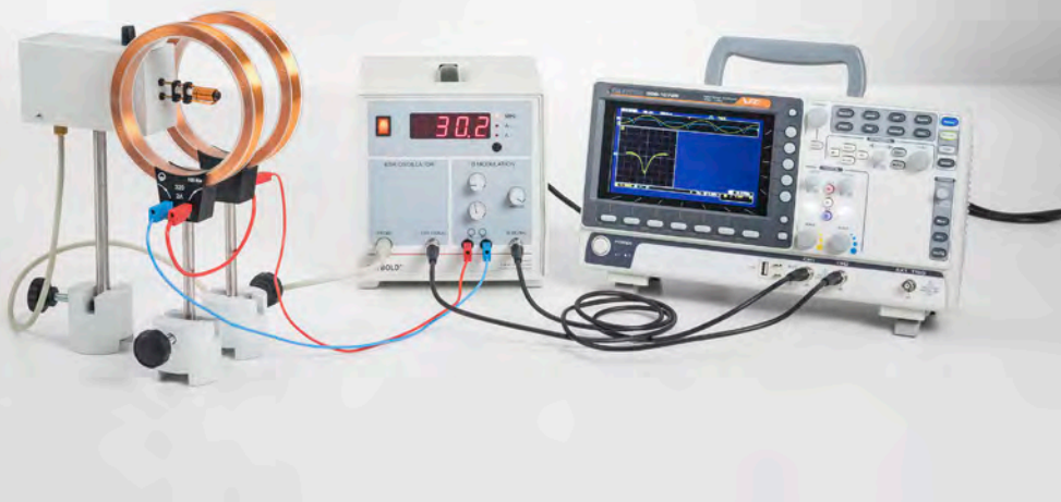
Electron spin resonance at DPPH - determining the magnetic field as a function of the resonance frequency (P6.2.6.2)
