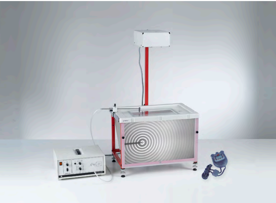
Exciting circular and straight water waves (P1.6.4.1)
