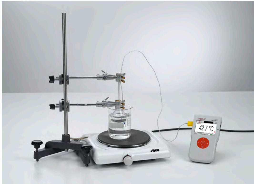
Determination of volumetric expansion coefficient of liquids - Measuring with Mobile-CASSY (P2.1.2.2)
