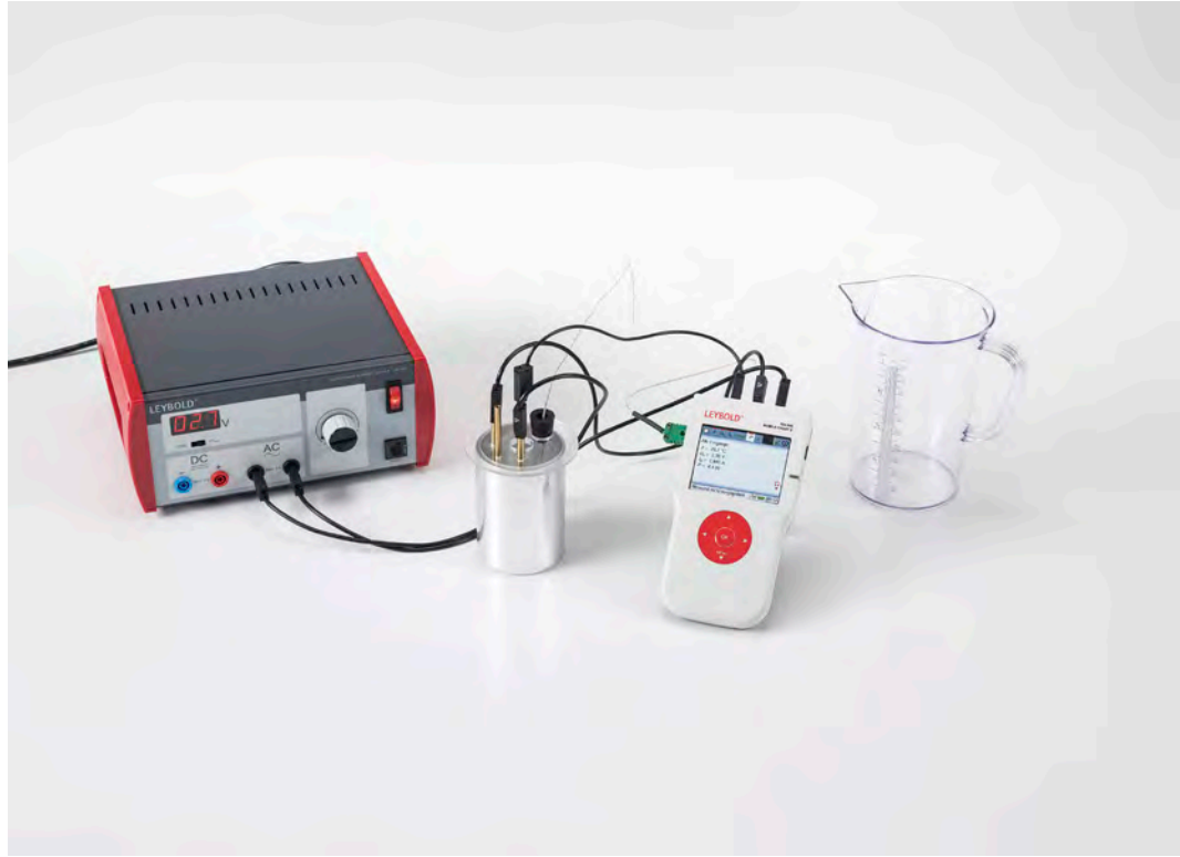
Determining the heating power of an ohmic load in an AC circuit as a function of the applied voltage (P3.6.6.1)
