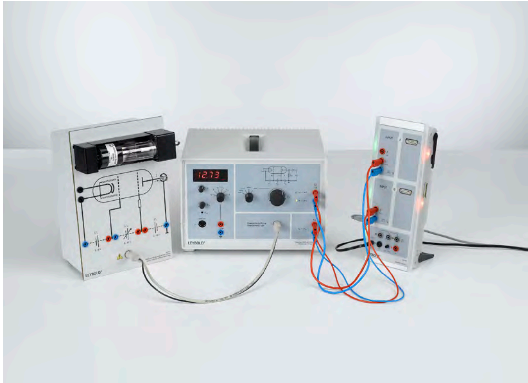
Franck-Hertz experiment with neon - Recording and evaluation with CASSY (P6.2.4.4)
