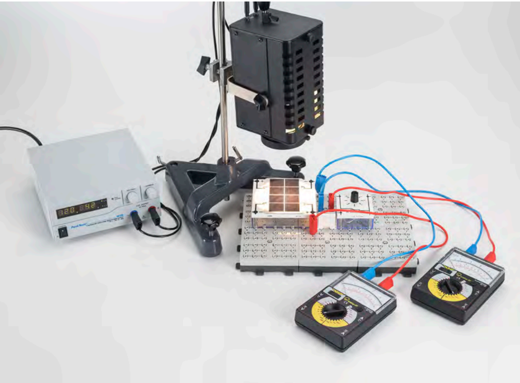
Recording the current-voltage characteristics of a solar battery as a function of the irradiance (P4.1.1.3)
