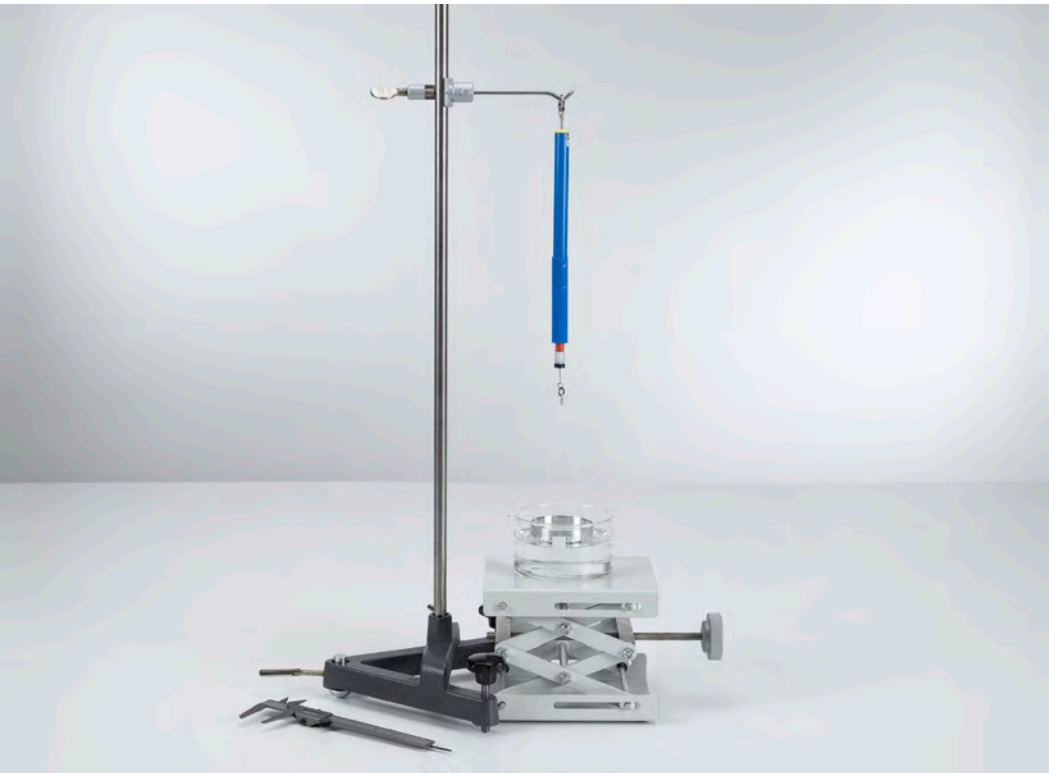
Measuring the surface tension using the „break-away“ method (P1.8.4.1)
