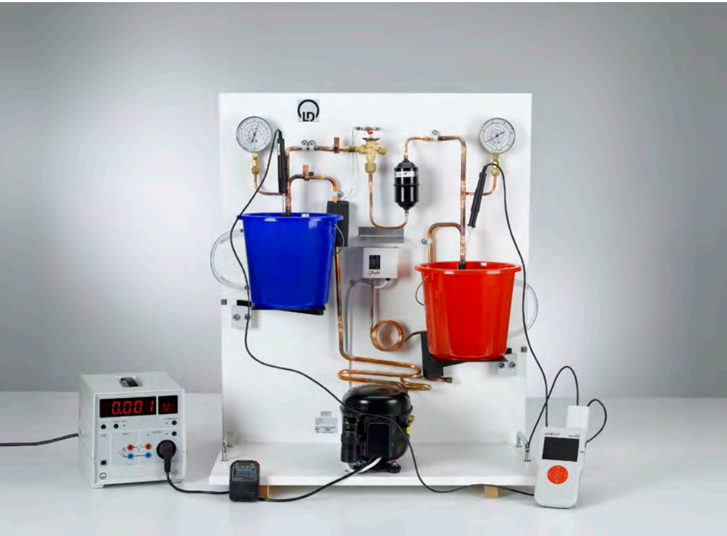
Determining the efficiency of the heat pump as a function of the temperature differential (P2.6.3.1)
