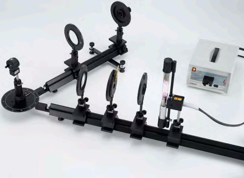
Observing the splitting of the Balmer series on deuterated hydrogen (isotope splitting) - Observing the line splitting with a telescope setup (P6.2.1.5)
