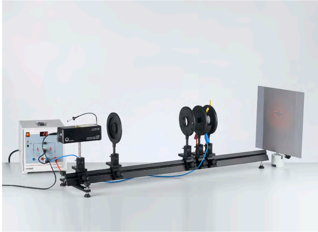
Demonstrating the Pockels effect in a conoscopic beam path (P5.4.5.1)
