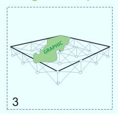
Graphic attaches to frame with velcro. Start in one corner and move on to the next.
