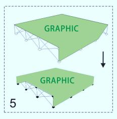
Pull end caps down to corner of frame and attach. Then attach other corner. Afterwards, repeat on opposite side.
