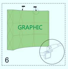
Attach the spot lights to the 2 mounts on top of the display stand.
