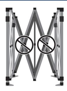
Be careful of the scissor sections of hardware as they are a pinching hazard.
