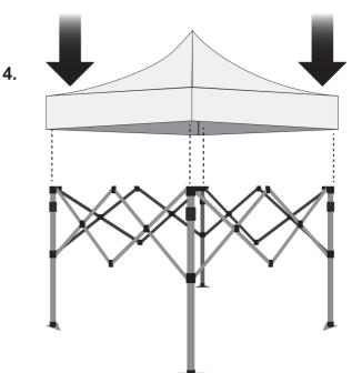
Unpack canopy graphic. Place on top of frame. Align canopy corners with hardware corners and fasten together using the velcro.
