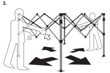
Standing across from each other, two people shoud use the center "V" of the hardware and lift up while stepping back. This will expand the frame. Stop when the frame is roughly 5 feet wide.
