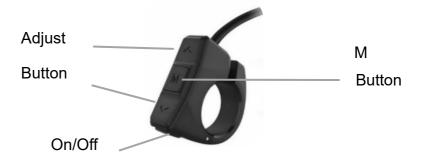
Short Press: Press the button and soon released, while the button is released, the function activated accordinglyLong Press: Press the button and hold, when the hold time exceeds the setting time(generally 2 seconds), the function activated accordingly.
