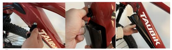
Remove battery Step 1: Turn the key into unlock position. Step 2: Rotate the battery lock as above photo shows. Step 3: Take out the battery with both hands.
