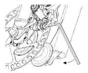
Always check that both your front and rear brakes are properly adjusted before riding your bike. Squeeze your brake together and slip the cable into the through. You may need to adjust the cable length by loosening the nut and sliding the cable through to the proper position. Retighten the nut to hold the proper position.
