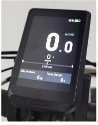
Long press the " $\bigcirc$  button" on display to switch on the LCD, and press "+" and "-" button to change assist levels. Short press the "M" button to change info on the screen.
