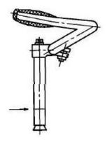
Check that the forks and the handlebars are facing forward and straight. Stand at the front of the handlebar, put the front wheel in between your legs and hold the handlebar. Adjust the handlebar and the body of the bicycle to form an angle of 90° (see the picture).
