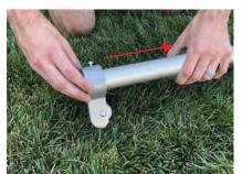
STEP FIVE: Place the pulley topper back on the top of the pole
