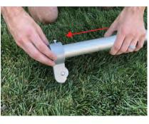
STEP TWO: Remove the pulley top of the flagpole
