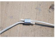
STEP TWO: Take the rope ends and insert into the connector. Once inserted, smash the connector with a hammer to secure the rope ends.
