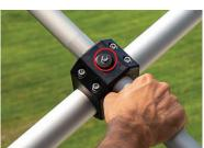
STEP THREE: Center the yard on so there is equal distance on both sides Tighten the front bolt on the yard arm connector to secure the yard arm left to right. \*\*Do not over-tighten
