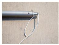
STEP ONE: Thread rope through one side on the yard arm, directly through the hole. Repeat on the opposite side.
