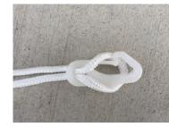
Loop part of the rope and thread through the bottom hole in the clip. Take the looped rope and wrap over the top of the clip.
