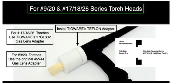
Remove the original Insulator & Install TIGWARE's Teflon Insulator
