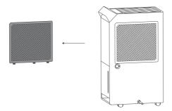
The filter can be removed for cleaning from the buckle on the left side plate and easily installed by inserting the fastener into the slot.
