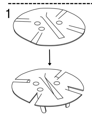
Using your fingers or pliers, bend the 4 tabs 90 degrees so that they point straight down. Then slightly bend the center tab approximately 45 degrees
