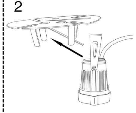
Slide the loop of the light through the center tab
