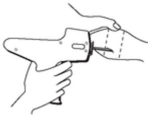
Fig. 2 - Rear View of the Bovine Ear Showing the Site for Insertion of the Implanter Needle.
