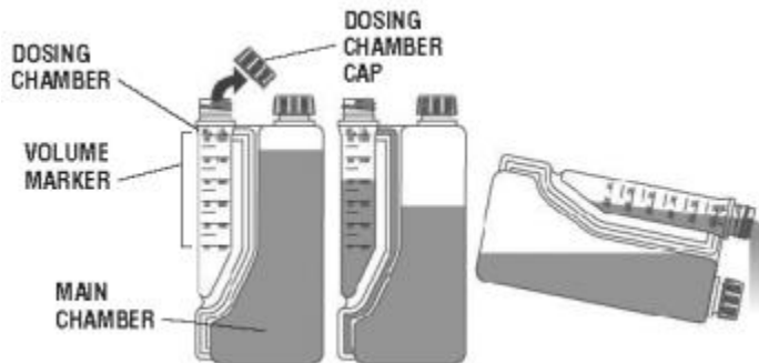
Figure 2. Squeeze-Measure-Pour System (16.91 fl oz/500 mL and 33.81 fl oz/1 L Bottles) Large Conventional Containers (84.54 fl oz/2.5 L and 169 fl oz/5 L Bottles and 338 fl oz/10 L Cubetainer)
