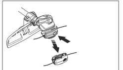
2. Pull out the line chute assembly.
