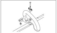
2. Move the spacer into the slot of the loop handle.
