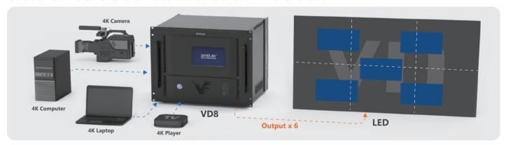
Solution 4: Connect to LED, LCD or projection screen in matrix mode
