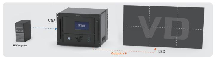
Solution 2: Multiple inputs and outputs in pixel to pixel splicing mode
