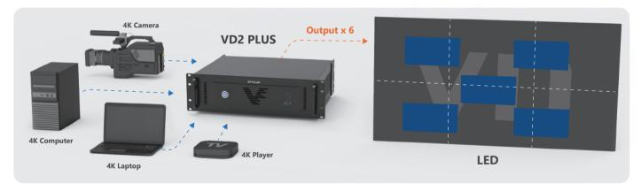
Solution 4: Connect to LED, LCD or projection screen in matrix mode
