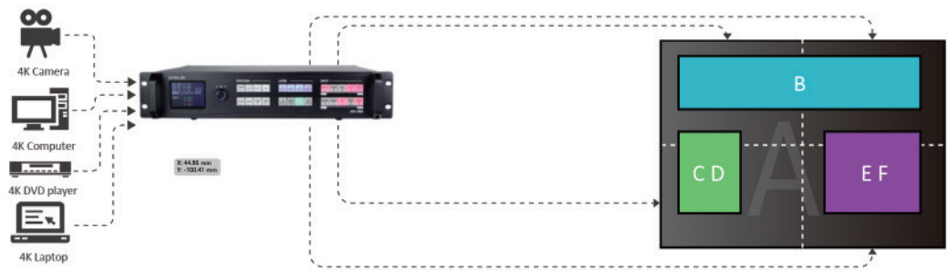
Application 2: Realize 6-windows display after splicing
