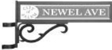
item# TSB-201 for use with 3" O/D round poles TSB201-624: holds 6" x 24" Street Blade Scroll: 16" long, 5 1/2" high
