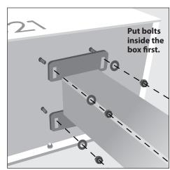
2. Use the Four Screws to attached to 3. Attach the box to the pole with the four included 7/16" bolts, washers and nuts using your 7/16" Socket or Crescent Wrench. Please Note: make sure both doors are in the lock positon, that way the doors will not swing and damage the finish of the doors. This can happen when installing the pole into the ground.
