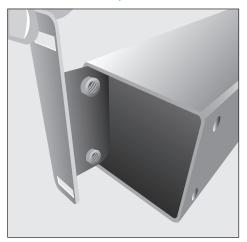
1. Insert brackets to line up with the side holes.
