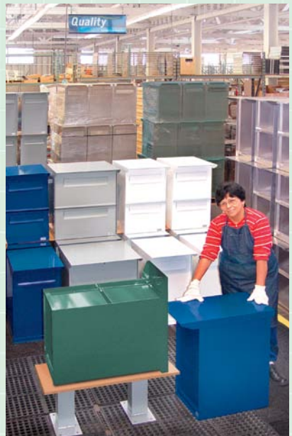
Final inspection of pedestal drop boxes
