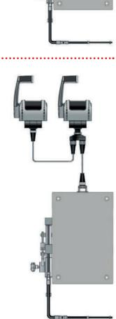
4500 SERIES SYSTEM FOR USE WITH SINGLE STATION CONTROL, TWIN ELECTRONIC ENGINES (4-20 mA) AND MECHANICAL GEARBOX
