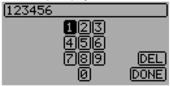
Fixed ID: The Fixed ID sets a unique code to ensure that the transmitter will only bind to a specific model. This is useful to ensure that the transmitter is not accidentally bound to the wrong model.
