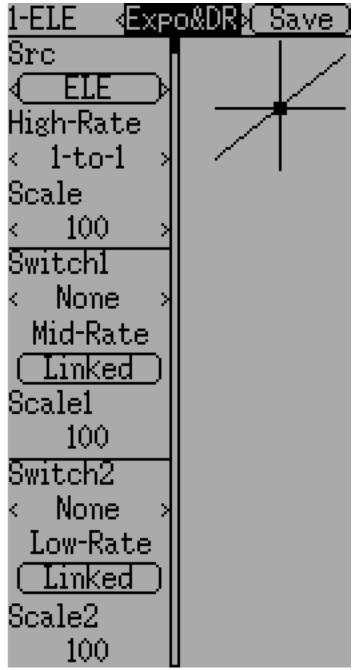
Selecting a value for Switch1 or Switch2 will activate the corresponding section. Each section can either have a 'linked' curve (curve is the same as the 'High-Rate' curve) in which case only the scalar can be modified, or alternatively can have an independent curve definition. Pressing the 'Mid-Rate' or 'Low-Rate' button for a given switch will toggle between linked and independent curves.
