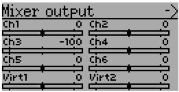
The channel monitor screen allows the user to see the values of each channel as output by the transmitter. Channels without mixers will not be displayed. Channel output displayed is the value based on minimum / maximum values as well as scaling.
