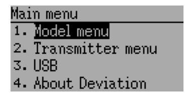
The main menu selections of the Deviation firmware are accessed by momentarily pressing the ENT button on the bottom right of the transmitter. The main menu consists of the following four options: Model menu, Transmitter menu, USB and About Deviation.
