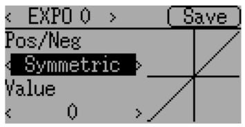
For the Expo curve, the controls allow independently configuring the shape of the curve for values greaterthan or less-than zero.
