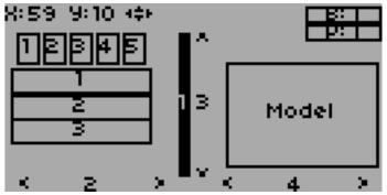
Pressing and holding the ENT button from the model configuration page will switch to the object position screen. Each of the visual objects can be selected using the UP/DN buttons. Pressing ENT again will allow moving the placement of the selected object. The UP/DN/L/R buttons will move the selected object on the screen. Press EXT once to exit move mode, and again to go back to the main page config menu.
