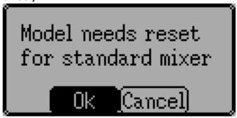
Mixer GUI: Defines which graphical user interface (GUI) to use for this model. The 'Advanced' GUI is the default for Deviation. The 'Standard' GUI is only available for Helicopter models and more closely resembles the stock GUI.
