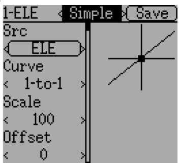
The Simple mix type is the simplest manner of defining a channel. It allows defining a primary-input (stick, switch, or other channel), and applying a curve or function to that input. The result can also be scaled or have an alternate zero-offset. You cannot use a toggle or switch to activate or deactivate this setup.
