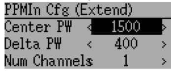
Deviation has the ability to use PPM input signals from an external source (such as an FPV setup). To configure this mode, set the PPM In mode to 'Extend' in section *Model setup (Std & Adv GUI)*.
