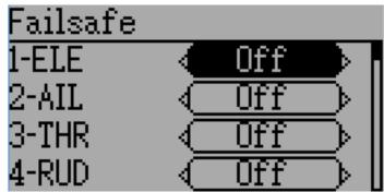
The fail-safe page is used to configure the fail-safe value for each channel (if the protocol supports this feature)
