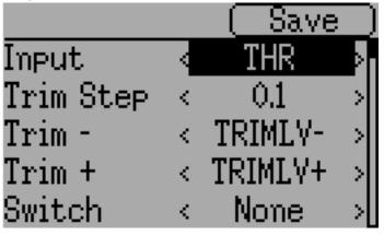
The trim-step defines how sensitive the trims are to input. The maximum number of trim steps is +/-100. So a step size of 0.1 will allow a full +/-10% of trim adjustment on the servo.
