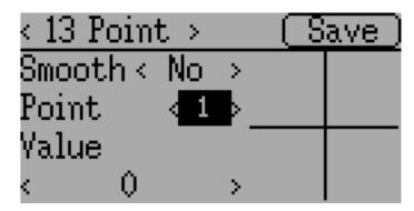
For the Multi-point curves, each point can be individually set. Points are set by choosing the point number and then choosing a value. The minimum number of points allowable is 3 the maximum number of points is 13. Enabling 'Smooth' will apply a smoothing function rather than connecting points via straight lines.
