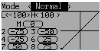
The throttle curve page allows defining a piece-wise linear curve for the throttle channel. Different curves can be selected for each flight-mode. Each point value can be enabled to be interpolated from the points surrounding it.
