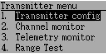
The configuration page defines various transmitter functions. It is entered from the main menu via 'Transmitter menu' followed by 'Transmitter config'. Please note that all screens in this section show the Deviation default settings.
