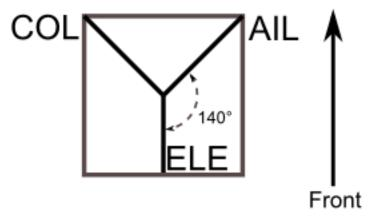
140 (3 Servo): Fundamentally, the servo operations of 140° swash-plates are almost the same as 120° swash-plates. However, the servo arrangement for elevator operation differs. 140° swash-plate CCPM offers smoother operation of the combined servos and an equal cyclic rate all around. On a 120° setup, the left/right cyclic is slightly faster than the fore/aft cyclic.
