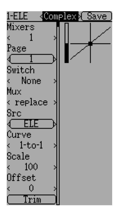
The Complex mix type unlocks the full power of the mixer system. For a given channel, any number of mixers can be applied to affect the final result. Each mixer is applied based on whether the specified switch is active, and can either replace, add to, or multiply to the previous mixers for this channel. Using this system it should be possible to define an output channel as a combination of any number of inputs.
