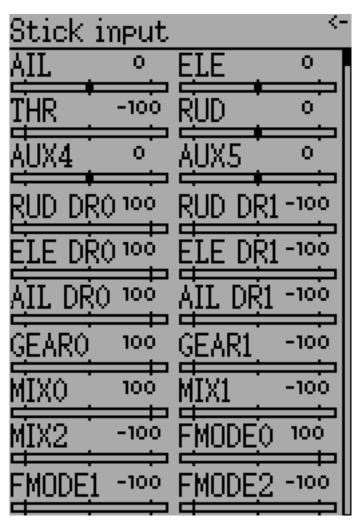
The input monitor screen shows the values associated with the current position of the control points. The values shown are a percentage of the total range of the controls based on a -100% to +100% scale.
