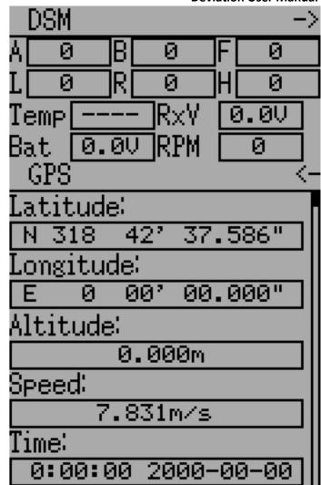
The following fields are available in DSM2 Telemetry. Note that a dedicated telemetry module and additional sensors are needed to capture this data
