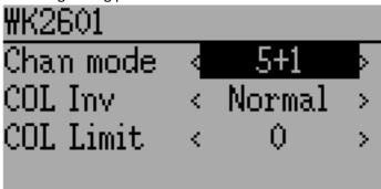
The WK2601 protocol also supports additional options. These are accessed by pressing the Protocol spinbox when Wk2601 is shown:
