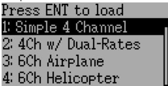
The Deviation firmware supports user-customizable predefined templates. By Selecting 'Template...' within the File spin-box from the Model page.
