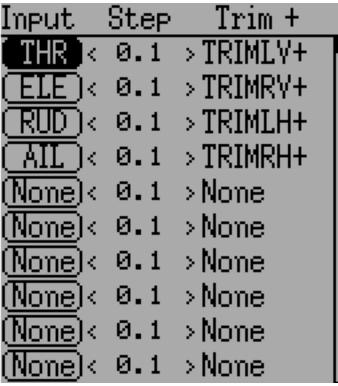
The trim page allows assigning the trim buttons and trim step, as well as configuring buttons to work as virtual inputs (see *Using a Trim as a Virtual Switch*). It is accessed from the main menu via 'Model menu' followed by 'Trims'.
