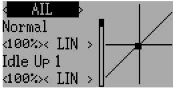
The dual-rate and expo page allows configuration of curves for the Aileron, Rudder, and Elevator channels. Up-to 3 rates can be configured for each channel, and either a scaled-linear or exponential curve can be selected for each. The number of settings depends on the switch assigned to the dual-rates function on the Switch Assignment page (see *Switch Assignment*)
