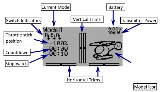
Current Model: The name of the current model. Clicking the label will open up the Model Load page. The model is configured from section *Model setup (Std & Adv GUI)*.
