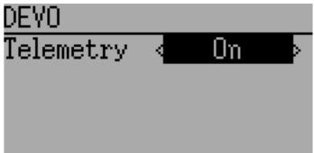
The DEVO protocol also supports enabling/disabling the telemetry capability. This option is accessed by pressing the Protocol spin-box when DEVO is shown.
