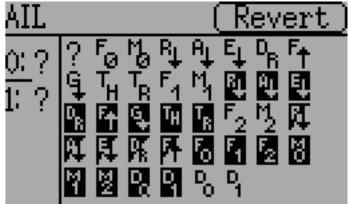
Pressing the 'Toggle' button on a toggle object allows selecting the related icons. Channels, sticks, and 2position sticks can have 2 icons. 3 position sticks (if any) can have 3 icons. Each of the 2 (or 3) icon states can be set to empty, defining that no icon is shown for this state. The Deviation firmware comes with several predefined icons to choose from.
