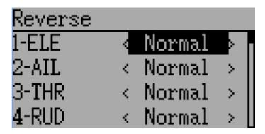
The servo reverse page allows quickly setting each channel to work in either normal or reversed mode. These settings are equivalent to the 'Reverse' setting on the Channel Configuration sub-page of the Mixer menu when using the Advanced GUI (see section *Channel configuration*)
