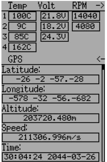
Certain protocols have the ability to transmit telemetry data back to the transmitter during use. Telemetry data may include, but is not restricted to, temperature readings, various voltage readings, motor or engine rpm, as well as GPS related information.
