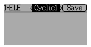
Cyclic1, Cyclic2, Cyclic3: The 3 outputs of the helicopter swash-plate mix. These will represent the 3 servos
