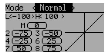
The pitch curve allows defining a piece-wise linear curve for the collective/pitch channel. Different curves can be selected for each flight-mode as well as for throttle-hold. Each point value can be enabled to be interpolated from the points surrounding it.
