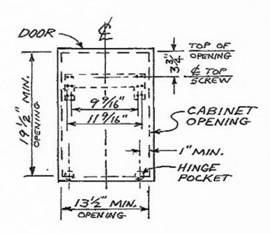
Install only one top screw on each side of frame, then test the motion to be sure that clearances are correct. After confirming clearances, install two more screws on each side.
