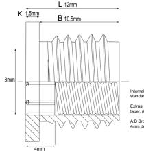
Internal thread: M8 standard pitch. Extrnal thread: 12mm external taper, (6 threads per 10mm) A:B Broached Hex Internal
