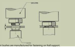
Anchor Rivet bushes are manufactured for fastening on frail support.
