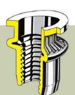
When setting, the flutes anchor the SERBLOC nut in the support, giving it considerable clamping strength. Torque. Resistance is higher than that of class 6.8 steel screw..
