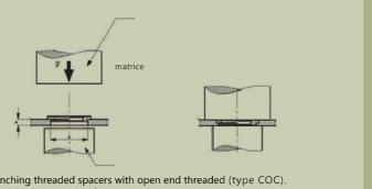
Self clinching threaded spacers with open end threaded (type COC). Inserted into a round hole.
