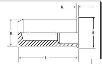
Round low profile head closed ended Rivetnuts for material up to 3.00 mm thick
