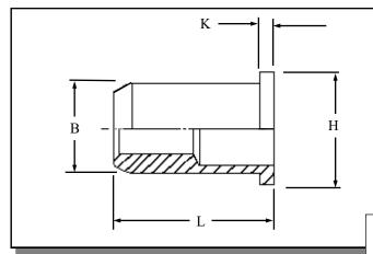
Round flat head open ended Rivetnuts for material up to .285" thick
