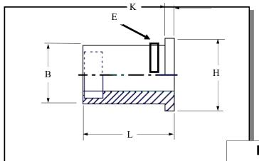
Round flat head open ended Rubber nuts for material up to 1.5 mm thick
