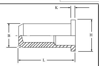
Round flat head closed ended Rivetnuts for material up to 5.50 mm thick
