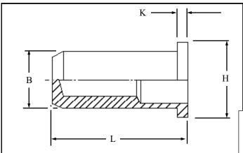
Round flat head closed ended Rivetnuts for material up to 3.00 mm thick
