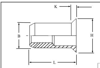
Round Countersunk head open ended Rivetnuts for material up to 4.50 mm thick
