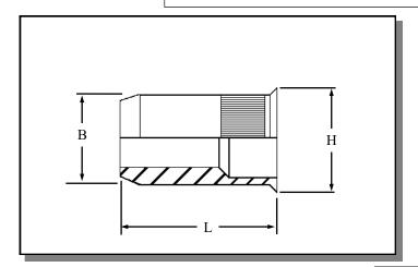
Knurled Round thin sheet open ended Rivetnuts for material up to 3.00mm thick
