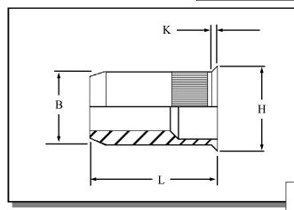
Knurled Round low profile head open ended Rivetnuts for material up to 3.00 mm thick
