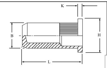
Round flat head closed ended Rivetnuts for material up to 3.20 mm thick
