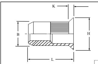
Knurled Countersunk head open ended Rivetnuts for material up to 4.50 mm thick
