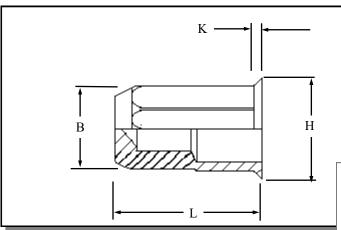
All Hexagon low profile head closed end Rivetnuts for material up to 3.0
