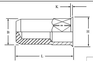
Hexagon low profile head closed ended Rivetnuts for material up to3.00 mm thick
