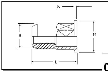
Hexagon flat head open ended Rivetnuts for material up to 3.00 mm thick
