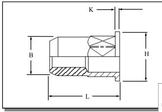
Hexagon flat head open ended Rivetnuts for material up to 3.00 mm thick
