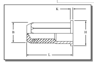
All Hexagon body flat head closed ended Rivetnuts for material up to 5.50 mm thick
