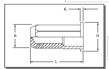
All Hexagon body flat head closed ended Rivetnuts for material up to 5.50 mm thick
