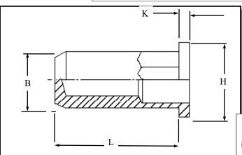
Hexagon flat head closed ended Rivetnuts for material up to 5.5 mm thick
