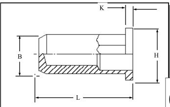
Hexagon flat head closed ended Rivetnuts for material up to 3.00 mm thick
