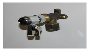
**Step 2:** This photo shows the braided line adapter fitted. All that is required is to unscrew the braided line off the mains supply and install the adapter. Once the supplied adaptor is fitted with the rubber washer inserted into the female thread of the adaptor, you can re-install the braided hose to the ½" male thread.
