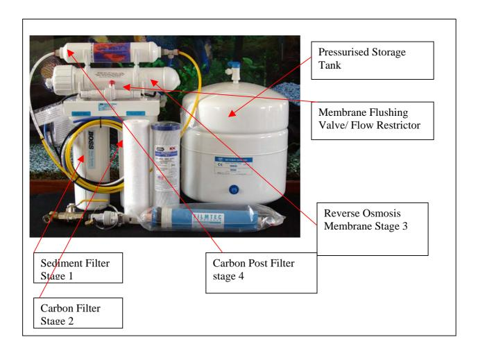
**Stage 1** Sediment pre-filter, this filter is a 1 micron polyspun sediment filter cartridge for mechanical removal of Grit, dust, Rust, mud, algae ect. This cartridge is normally replaced every 12 months but if dirty mains water is encounted more frequent change may be required.
