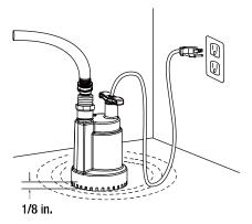
**NOTE:** After starting, the pump will lower the water level to 1/8 in. (3.2 mm) before losing suction. It will not pick up water less than 1/8 in. (3.2 mm) deep when running and will not operate successfully if started in only 1/8 in. (3.2 mm) of water.
