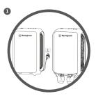
Disconnect the power supply, hold the two buckles at the bottom of the Front Cover, to take off the Front Cover.
