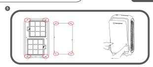
First, align the four pins on the Front Cover with the four holes on the unit. Then, slightly push the Front Cover, the magnetic parts will attract the Front Cover towards to unit body. The installation of Front Cover is completed.
