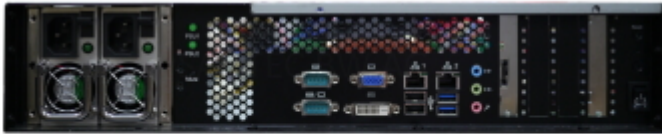
Redundant Power R2 Version
