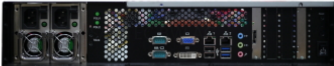
Redundant Power R2 Version
